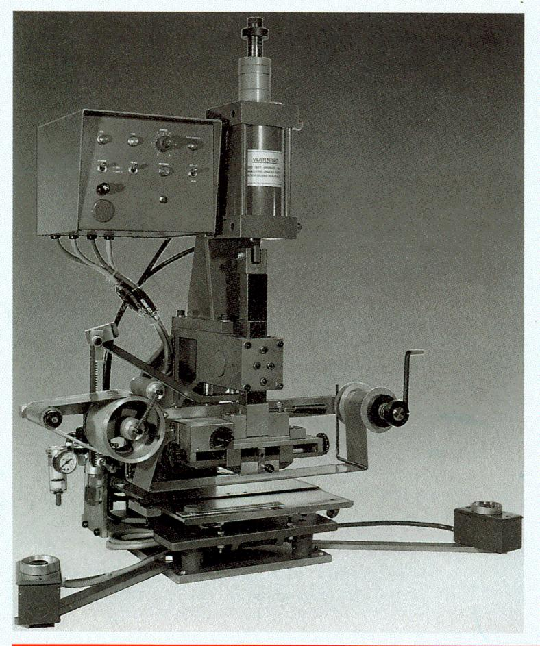
The Model 115A Air Operated Hot Stamping Machine is a versatile bench top machine capable of stamping many plastic items, vinyl items, medical products, pressure sensitive labeling materials, and can be equipped to do consecutive numbering.
